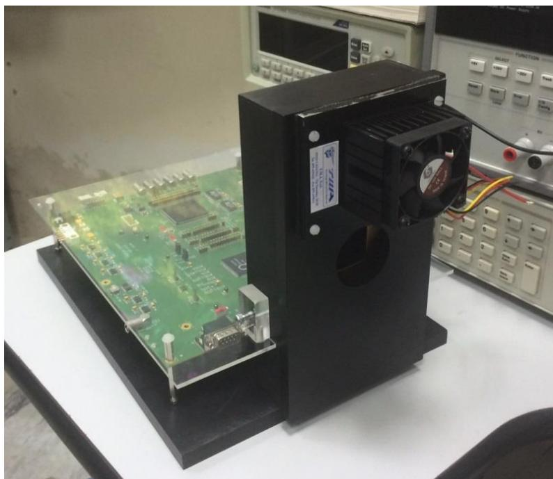
*Figure 4. CITIROC evaluation board and the black light-tight box with cooling system based on Peltier TEC.*
